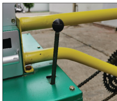
Figure 3. Clutch lever for shifting of drive.
