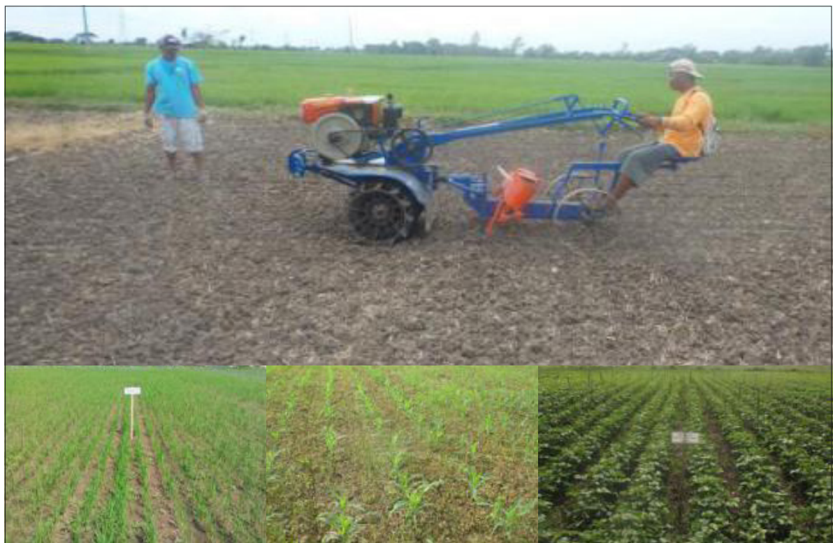
Figure 6. The MP seeder and established crops: (a) rice, (b) corn, and (c) mungbean.
