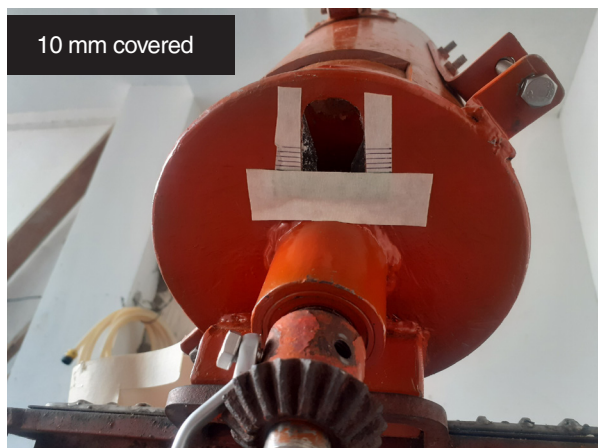
Figure 6. Improvised restrictor plate setting during testing.
