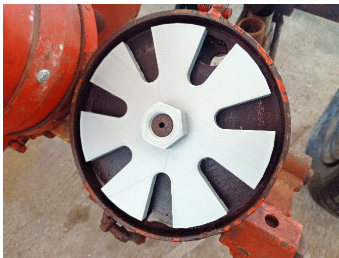
Figure 4. Slotted 10-mm-thick fertilizer plate for corn to dispense 465 kg/ha of complete fertilizer.
