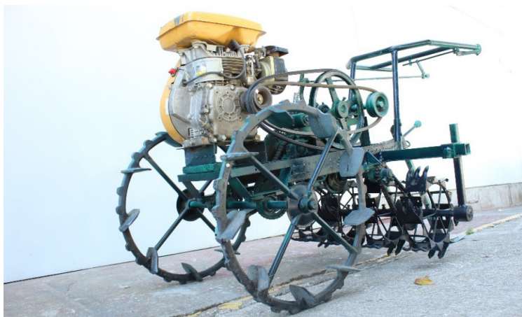
Figure 8. Final prototype of the 4-row mechanical weeder.
