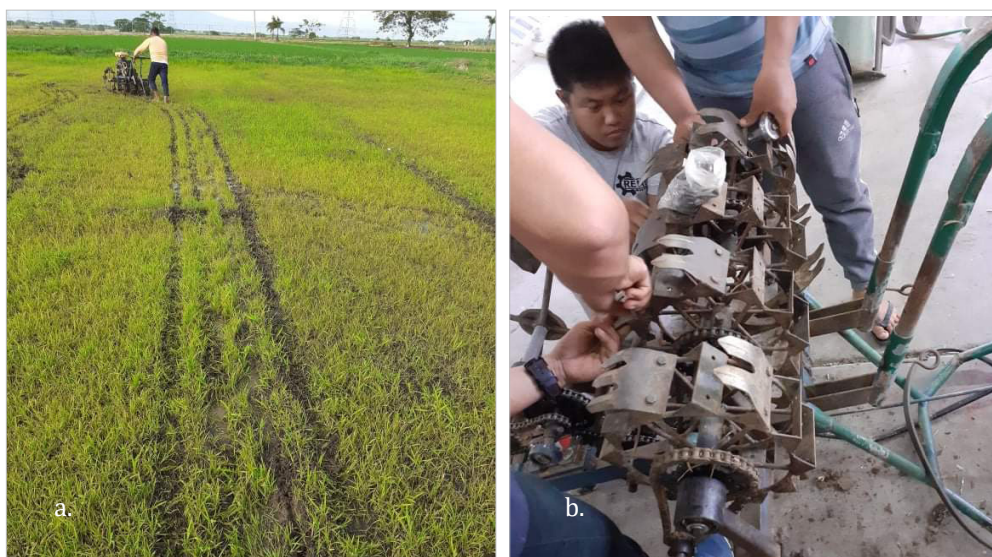
Figure 7. Mechanical weeder subjected to a.) field test and b.) fine-tuning.
