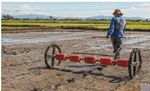
Sowing pre-germinated seeds using drumseeder
