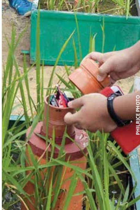
Capable of remote water-sensing, AutoMon PH operates through sensory objects and automatically gauges water level and alerts farmers via SMS.
