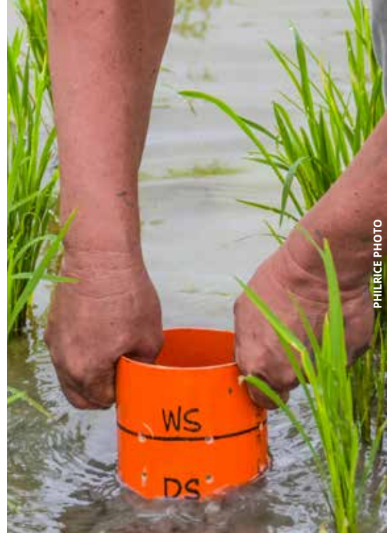
The observation well guides farmers in conducting the alternate wetting and drying technology, which can help save water by as much as 50 percent.
