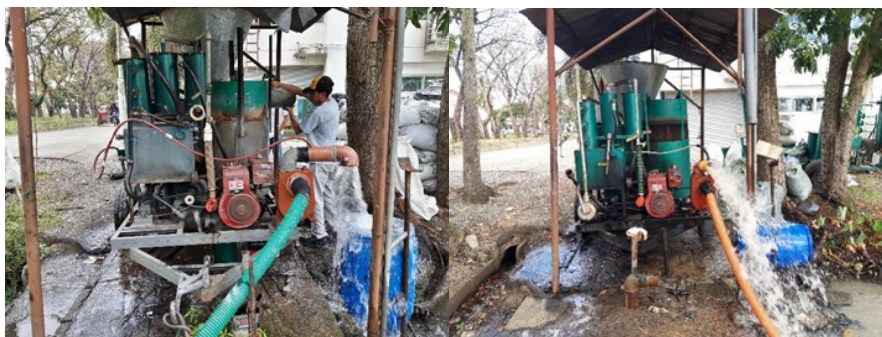
Figure 12. Performance testing of the rice hull gasifier engine pump system (RHGEPS) at open water source (left) and shallow tube well source (right).
