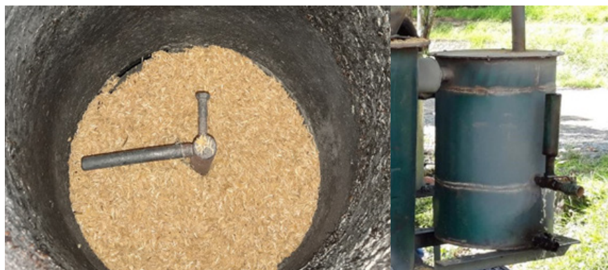
Figure 11. (Left) Simplified char scraper; (Right) primary gas cooler
