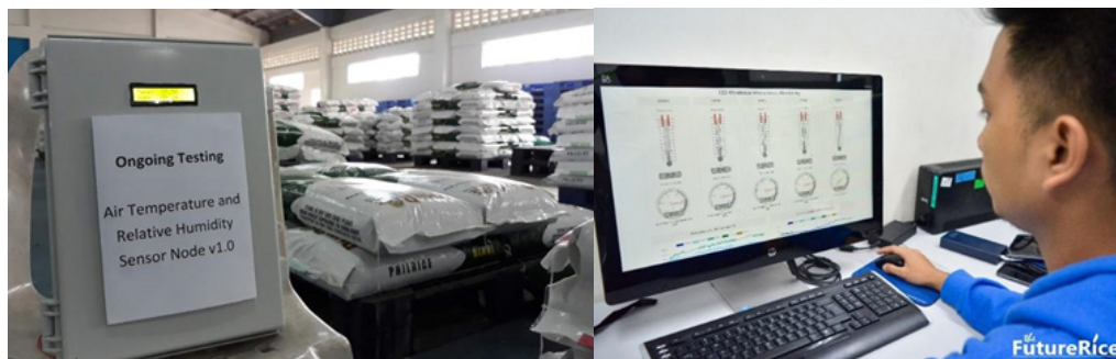
Figure 24. The microclimate sensing device installed at the CES seed warehouse (left) and the remote dashboard at the office showing real-time microclimate readings (right).
