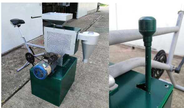
Figure 18. Improved prototype with electric motor (left) with dog clutch (right)
