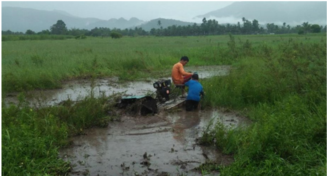
Figure 2. Actual testing of the prototype with plastic body in laboy field
