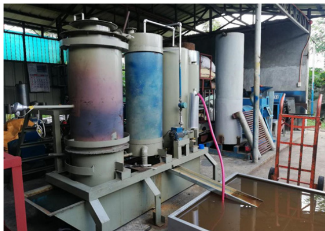
Figure 13. Rice husk gasifier system for single cylinder diesel engine currently being tested in San Rafael, Bulacan
