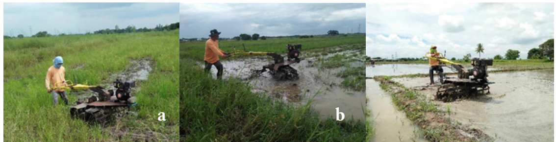
Figure 6. Testing of the prototype using rotavator, harrow, and riding-type leveler attachment
