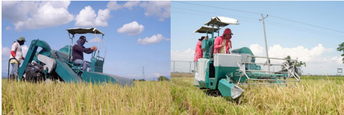
Figure 10. Actual field operation of stripper combine (left) and cutter bar combine (right)
