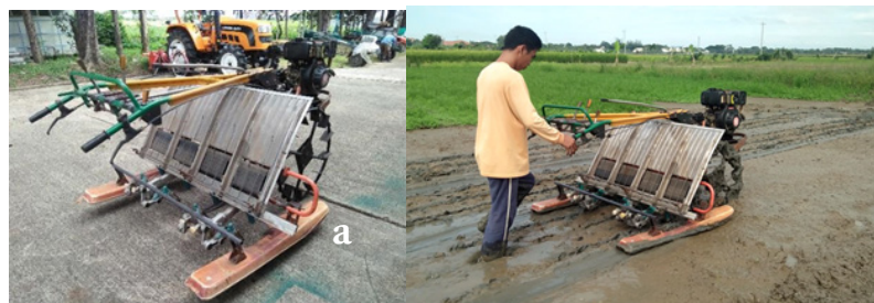
Figure 7. The fabricated prototype with rice transplanter attachment (left) while undergoing functionality test (right)
