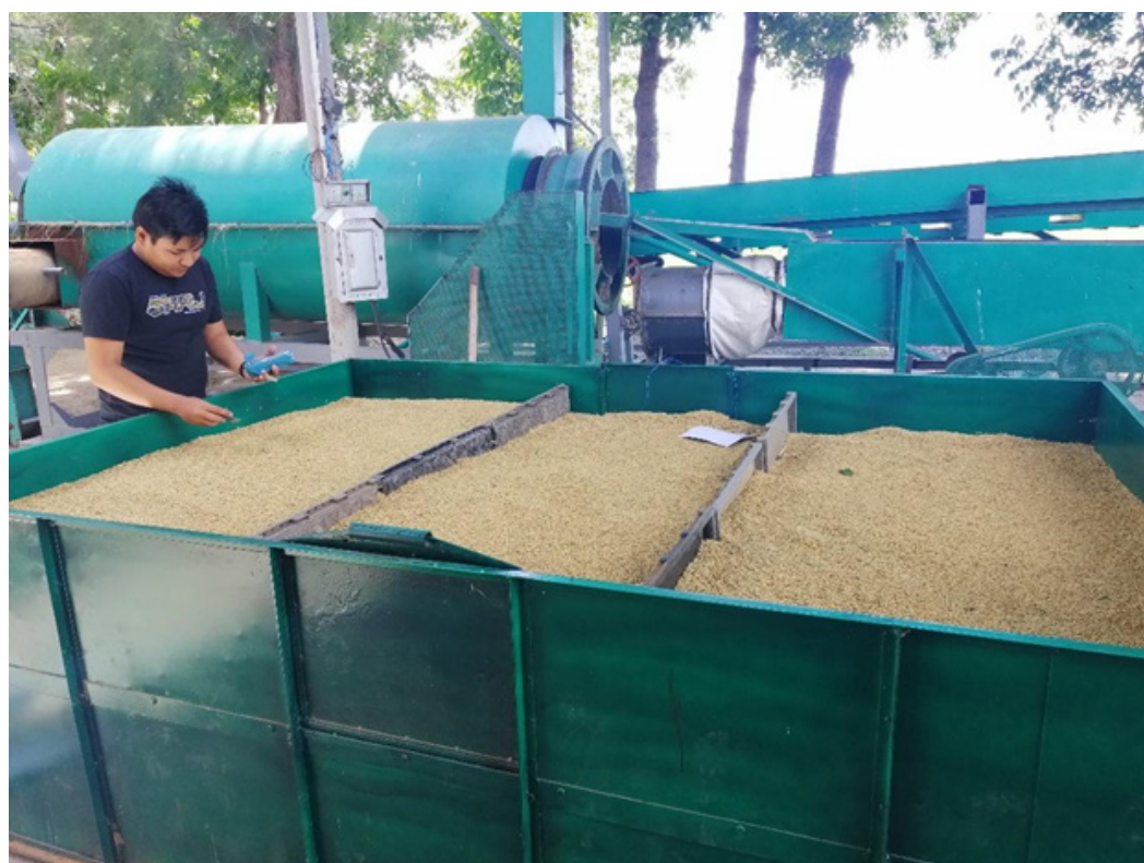
Figure 19. Mechanical (flatbed) drying of combine harvested samples (2019 DS)
