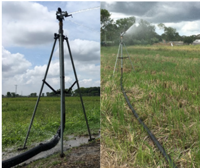
First prototype of the sprinkler system (left, Lay-flat hose) compared with the improved system (right, PE hose)
