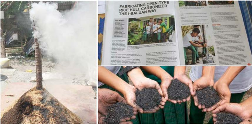
**Improvised open-type rice hull carbonizer.** The school was also noticed for fabricating their own version of the open-type rice hull carbonizer made of recycled paint and milk cans with rivet fasteners. A farmer from Nueva Vizcaya and a local businessman in their community liaised with our partner-teacher to learn the fabrication technique, and the process of producing CRH after they read the school’s story published in the June 2017 issue of *Agriculture Magazine*.
