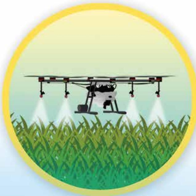
Drone sprayers vary on how they are operated. Some need to be fully operated using remote control while some allow for presets that let the drone fly by itself. Aside from technical considerations, operating it might require a permit from the Civil Aviation Authority of the Philippines (CAAP), depending on the drone characteristics like size and weight. For better information, drone operators should get in touch with CAAP.
