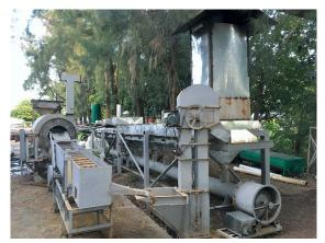
**Figure 12.** The combined rotary conduction and far infrared radiation paddy dryer.
