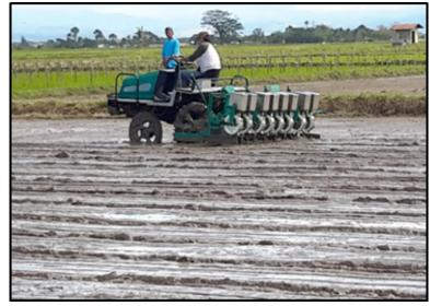
**Figure 22.** Improved riding-type precision seeder with 13hp gasoline engine 1800rpm-reduction type and power steering mechanism (January 27, 2016).
