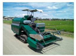
Figure 17. Combine harvester first prototype
