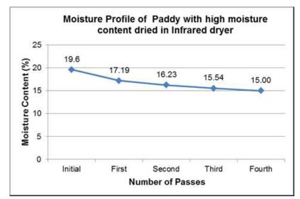
**Figure 15.** Moisture reduction curve of re-wetted paddy dried in the far infrared radiation dryer.
