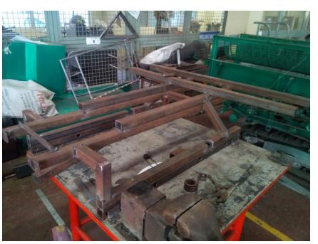
Figure 1. Undercarriage Frame and Chassis.
