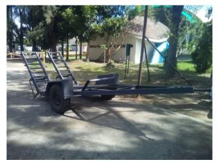
Figure 19. Tractor Trailer for 1.3 meter Rice Combine Harvester
