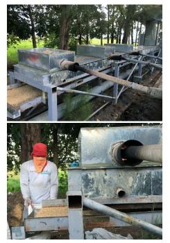
**Figure 13**. Three direct burners using producer gas from the rice husk gasifier heated the pumice (cement-ash mixture) surface emitter to generate far-infrared radiation.
