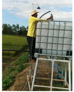
Figure 3a. Gathering discharge rate of the HRP at 2m elevation.
