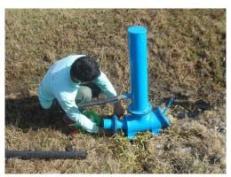
Figure 4. A 3" hydraulic ram pump from Tayum, Abra.
