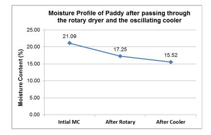
Figure 14. Paddy moisture reduction after passing through the rotary dryer and oscillating cooler.
