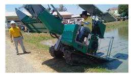
Figure 18. Combine harvester prototype climbing on dike.
