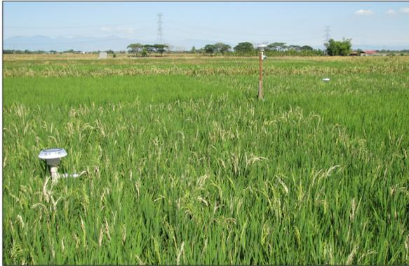
Figure 3. MINCER (Micrometeorological Instrument for Near Canopy Environment of Rice) installed at the start of the reproductive stage of the rice plant to record temperature and RH every 2 min for 24 h.
