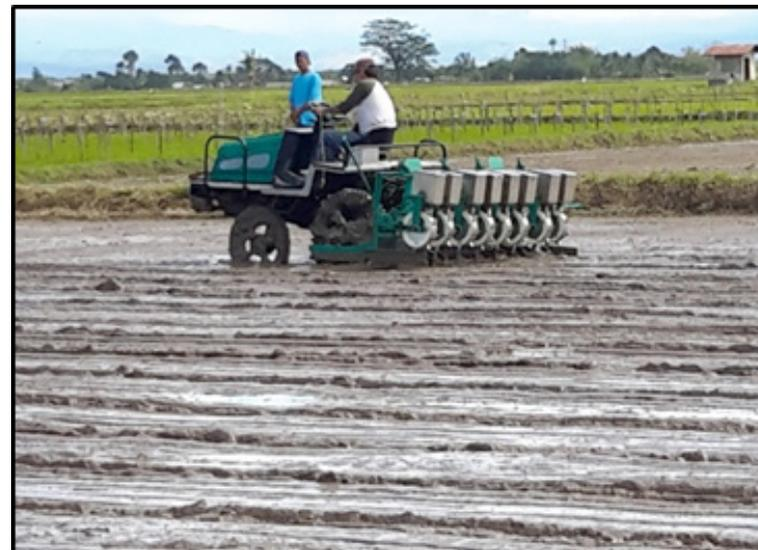
**Figure 22.** Improved riding-type precision seeder with 13hp gasoline engine 1800rpm-reduction type and power steering mechanism (January 27, 2016).
