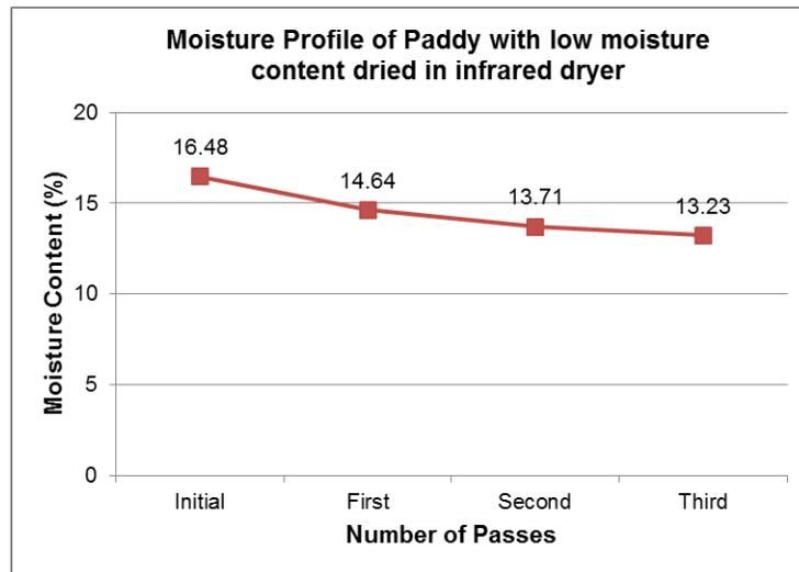
**Figure 16.** Moisture reduction curve of partially dried paddy completely dried in the FIR dryer.
