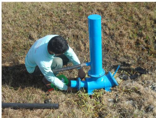
**Figure 4.** A 3" hydraulic ram pump from Tayum, Abra.
