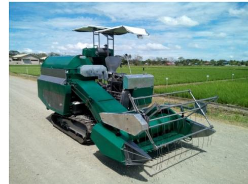
**Figure 17.** Combine harvester first prototype
