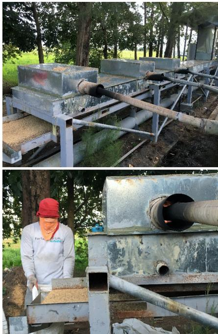
**Figure 13.** Three direct burners using producer gas from the rice husk gasifier heated the pumice (cement-ash mixture) surface emitter to generate far-infrared radiation.
