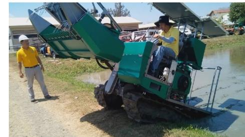
**Figure 18.** Combine harvester prototype climbing on dike.
