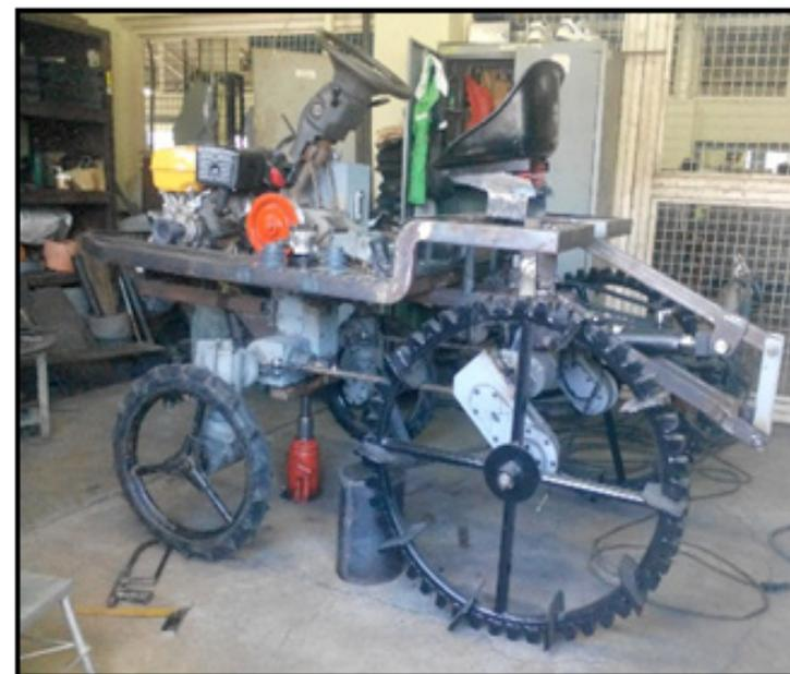
**Figure 23.** Assembly of improved prototype riding-type precision seeder.
