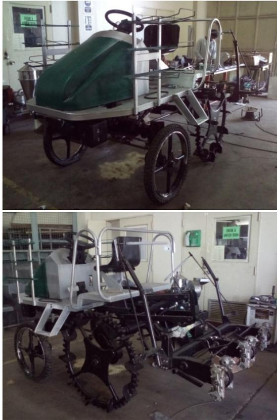
**Figure 21.** Local riding-type transplanter commercial prototype being assembled.
