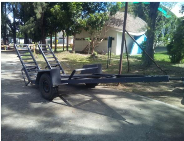
**Figure 19.** Tractor Trailer for 1.3 meter Rice Combine Harvester
