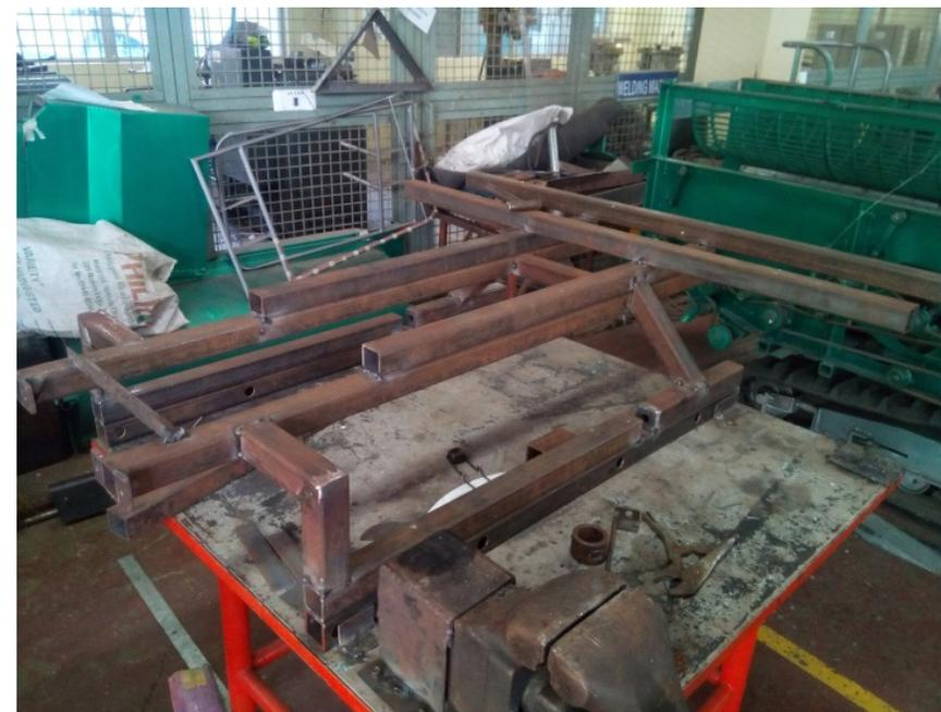
Figure 1. Undercarriage Frame and Chassis.
