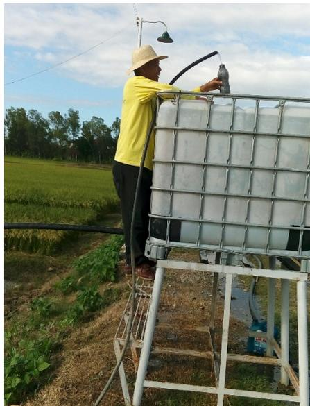
**Figure 3a.** Gathering discharge rate of the HRP at 2m elevation.
