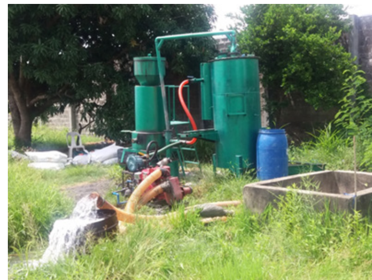
Figure 4. Actual field testing of the gasifier-pump at PhilRice's Palayamanan area using STW source.
