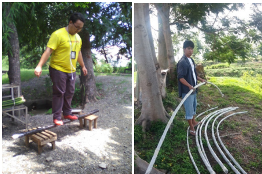
Figure 7. The improved prototypes of the basic construction unit: (a) the straight BCU (subjected to load using body weight), (b) the curved BCU.
