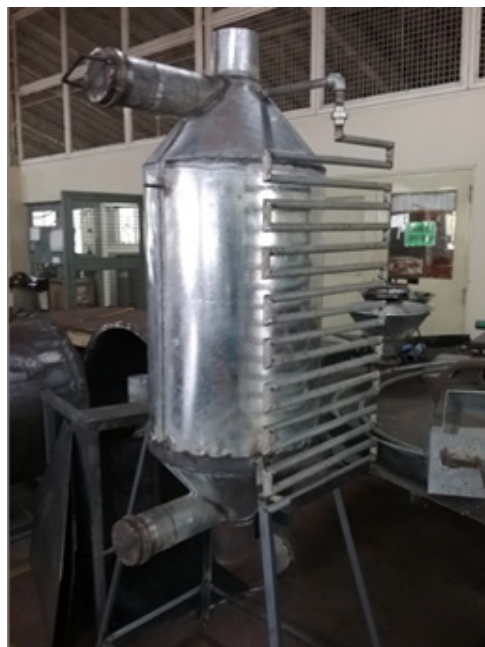
Figure 12. The carbonizer attachment for pyrolyzing biomass wastes for small scale power generation.
