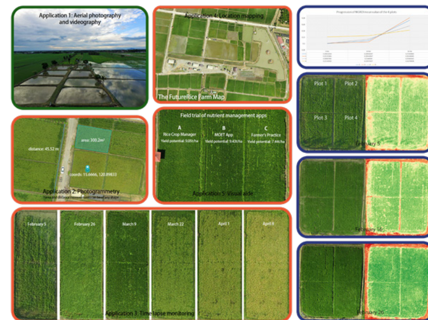
Figure 7. Drone-based aerial imagery applications using DJI Phantom 3 Professional quadcopter: (1) Aerial photography and videography; (2) Photogrammetry; (3) Time lapse monitoring; (4) Location mapping; (5) Visual aide; and (6) Vegetation index calculation.
