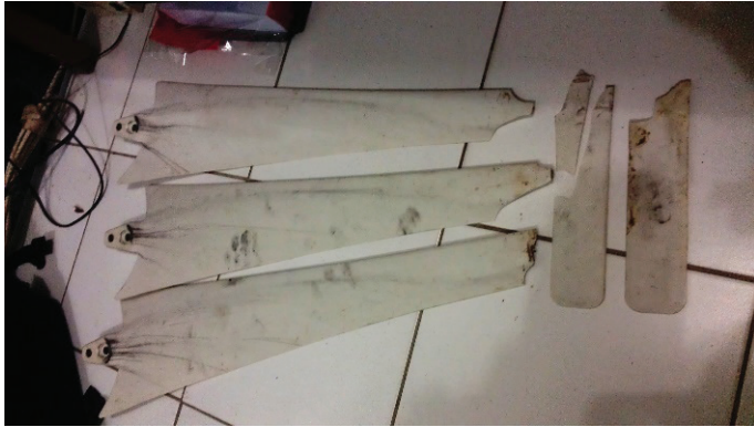
Figure 10. The turbine blade after typhoon “Egay”, July 2015.
