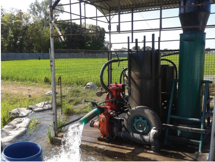
Figure 12. Ricehull Gasifier Engine-Pump system operation at PhilRice Baloc farm, DS 2015.
