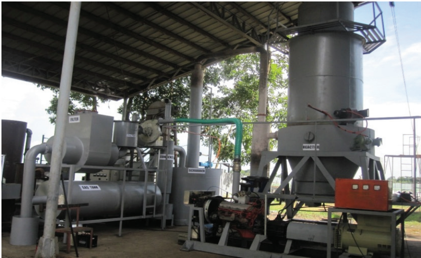
The 100-KW Rice Husk Gasifier
