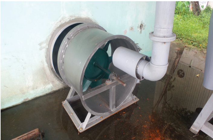
Figure 18. The s-vane tube axial type fan tested in a test duct system.
