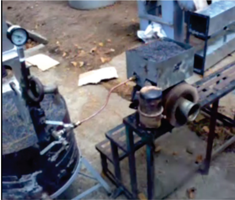
Figure 3. The ISG prototype coupled to a steam engine.
