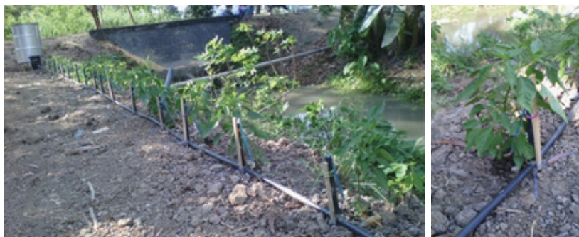
Figure 11. Initial field setup of the capillarigation system using cotton yarn as wick and green pepper as test crop.
