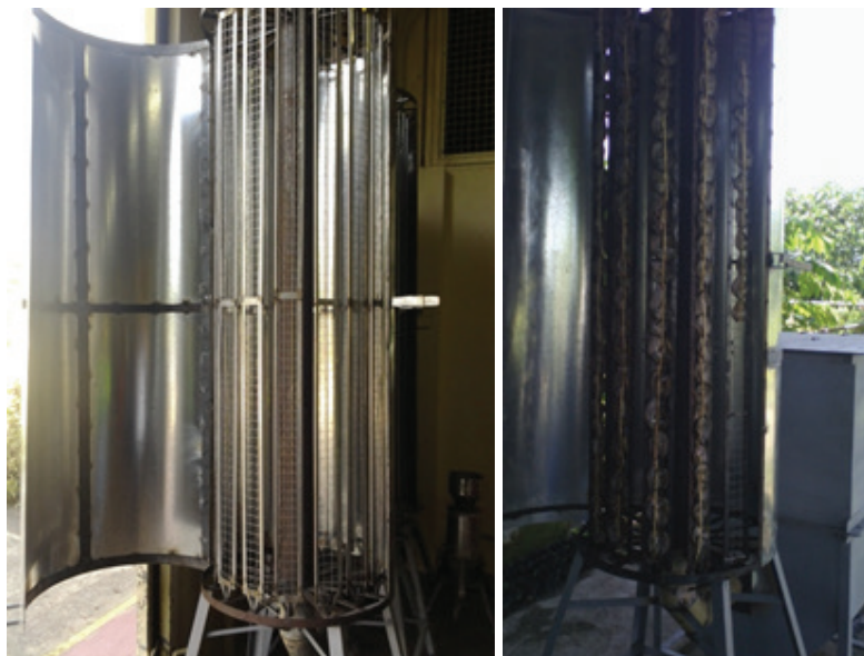
Figure 12. The multi-purpose dryer attached to the CtrRH carbonizer.
