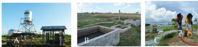
Figure 3. A) Solar powered water pump, B) Biogas digester, and C) Bioethanol powered water pump.
