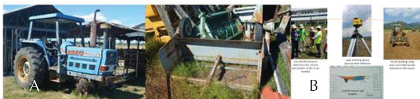
Figure 11. A) PhilRice laser leveler implements ready for re-activation and B) laser leveling process.
