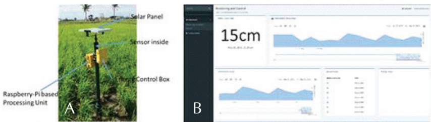
Figure 10. A) Components of the water level monitoring prototype model and B) Water level monitoring interface.
