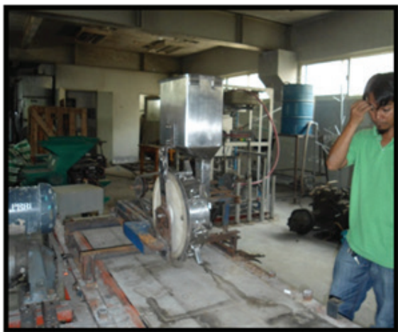
Figure 18. Laboratory testing of the seed metering device.
