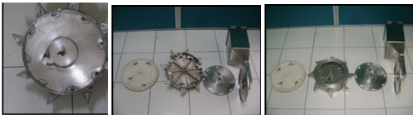
Figure 15. The seed metering device.
