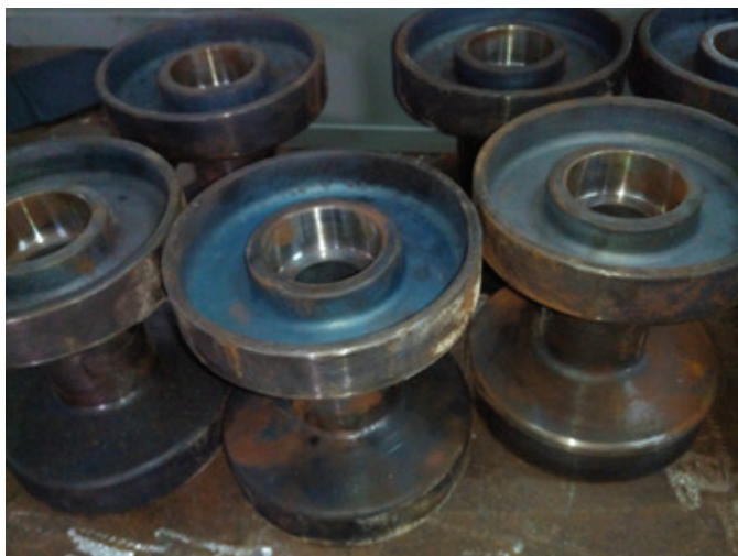
Figure 10. Undercarriage rollers fabricated by a MIAP member.
