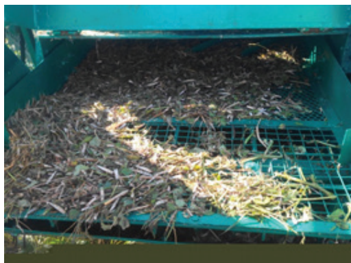
Figure 4. Matting of harvested materials on oscillating sieve.
