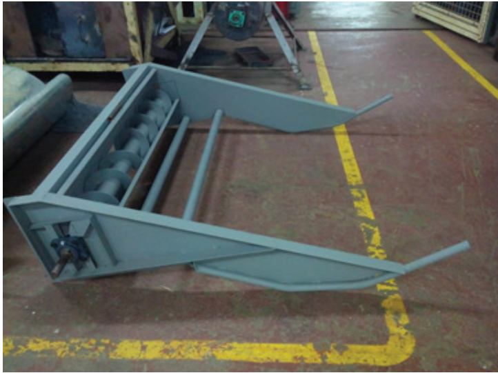
Figure 2. Intake auger inside the stripper header.
