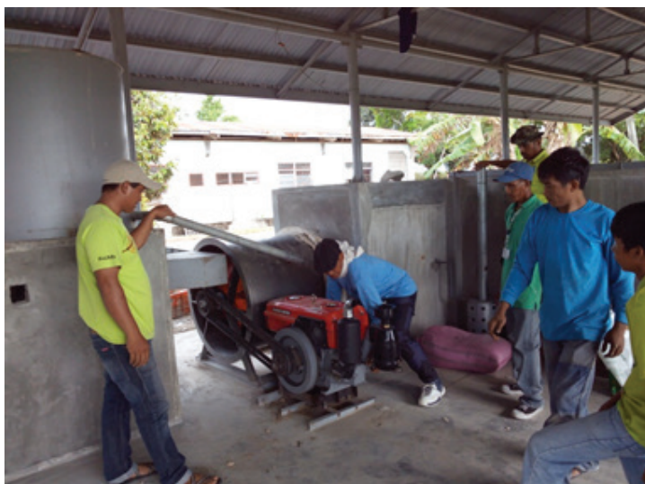
Figure 16. Testing of 8-ton reversible airflow dryer in PhilRice Midsayap.
