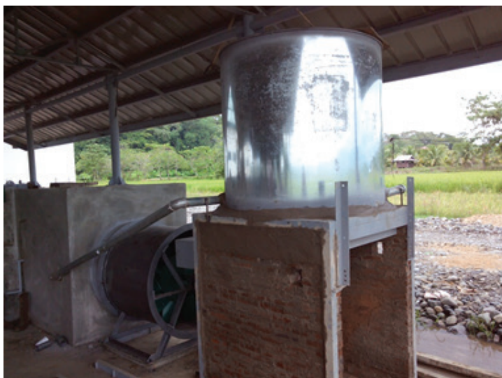
Figure 15. 8-ton reversible airflow dryer installed in PhilRice CMU.
