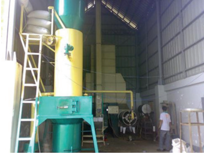
Figure 32. Final prototype of continuous flow rice hull gasifier as heating device for recirculating dryer.
