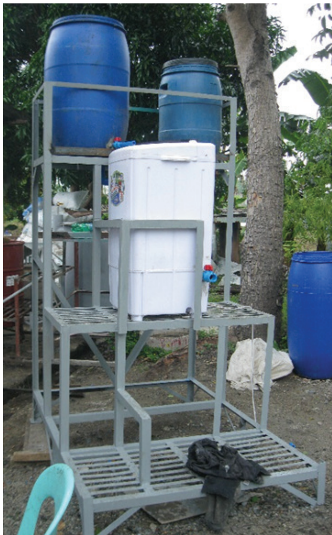
Figure 21. The prototype of a micro-processing plant for biodiesel production.
