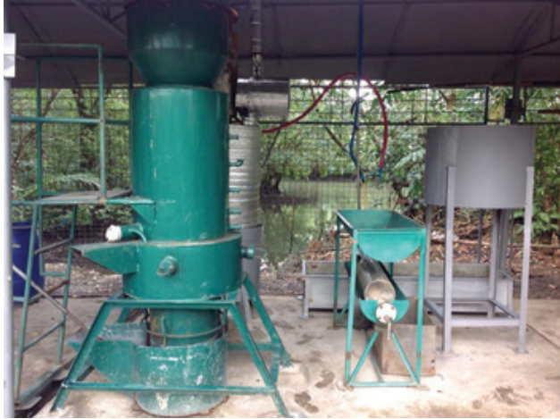
Figure 19. The hydrous bioethanol distilling facility installed in Infanta, Quezon.
