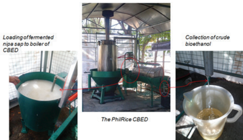
Figure 7. Distillation of fermented nipa sap using crude bioethanol distiller.
