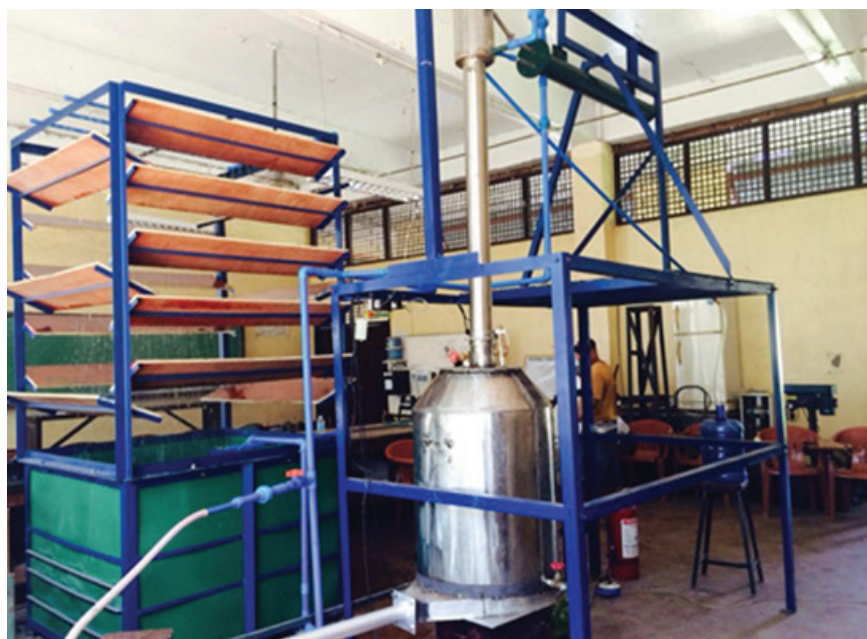
Figure 20. 200L capacity reflux distiller with improved furnace and cooling system.
