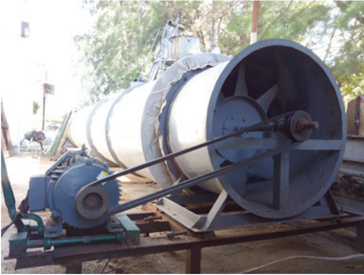
Figure 34. The s-vane tube axial type fan being tested in a test duct system.
