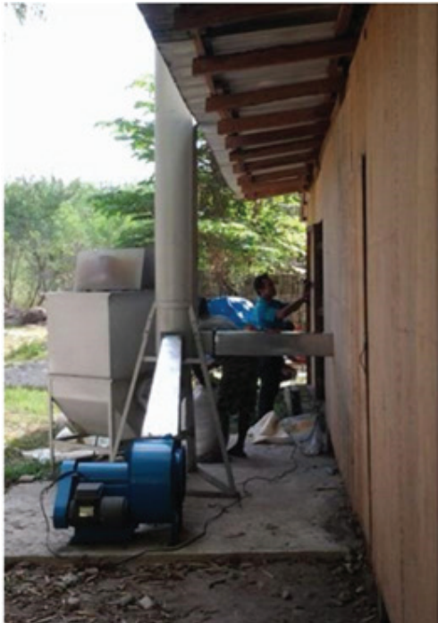
Figure 10. The carbonizer used as heat source in poultry brooding.
