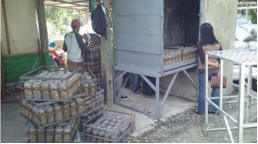
Figure 9. The 500-bag capacity mushroom pasteurizer.
