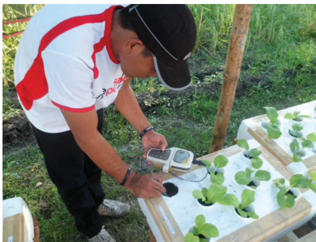
Figure 46. Measuring water concentration data using the Oaklon CON 400.
