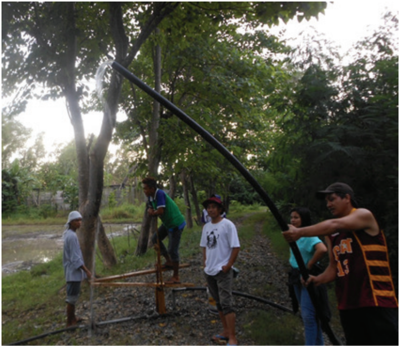
Figure 10. Treadle pump tested in Shallow Tube Well (STW).
