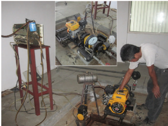
Figure 9. Brake dynamometer of 6.5 kenbo spark-ignition engine at PhilScat
