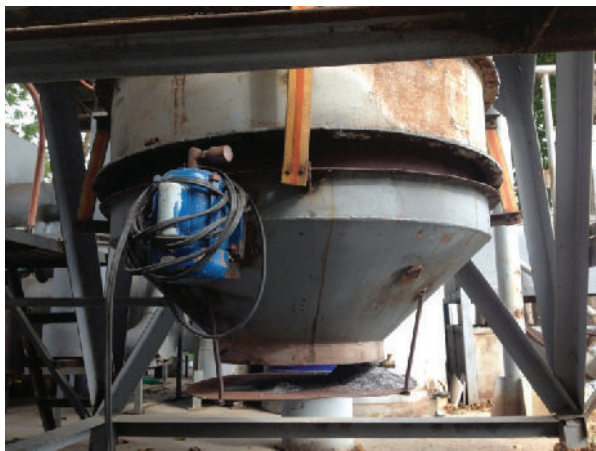
Figure 1. The modified CRH discharge of the 100kW gasifier reactor
