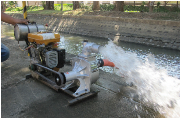
Figure 8. Water pumping using hydrous bioethanol as fuel
