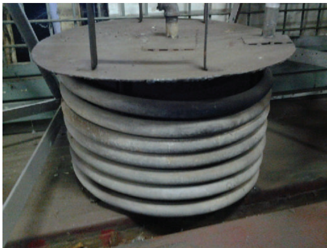
Figure 4. The prototype of the instant steam generator.
