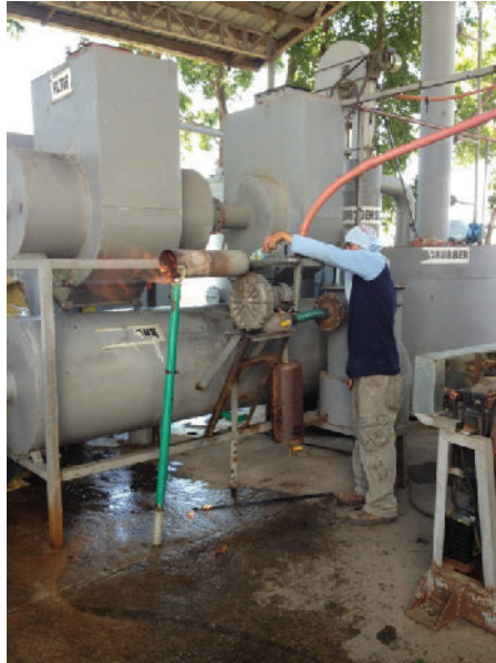
Figure 3. The 100kW gasifier during actual test
