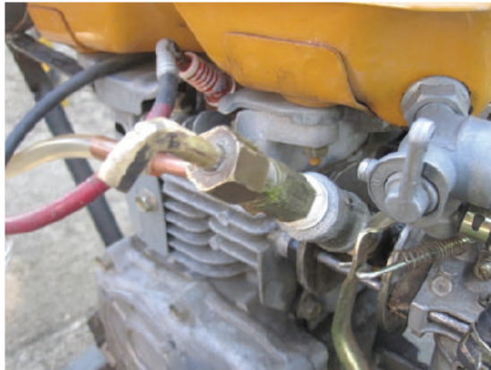
Figure 7. Fuel-feeding device attached to spark-ignition engine
