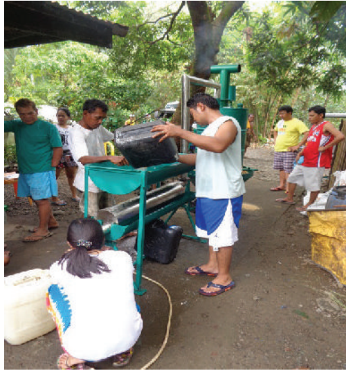
Figure 6. Field-testing of crude bioethanol distiller at Infanta, Quezon
