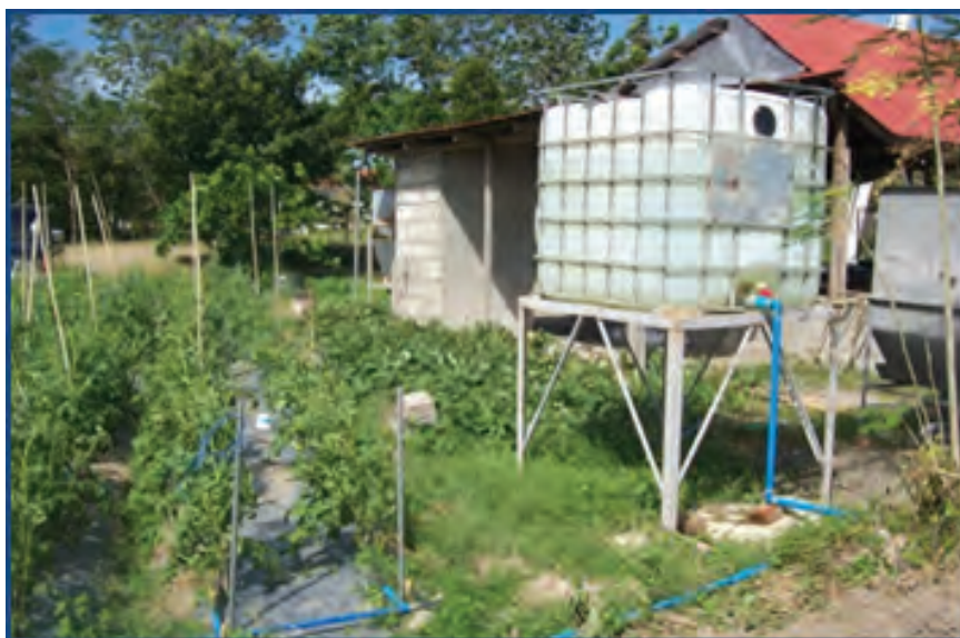
Figure 31. The carbonizer-pump set installed in a drip-irrigated tomato plot.
