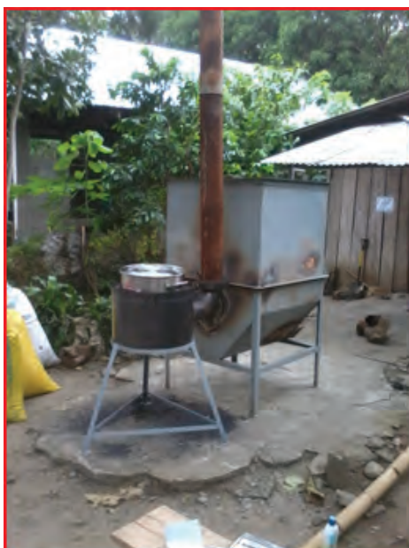
Figure 26. The heating chamber (attached to the CTRH carbonizer) undergoing water boiling test.
