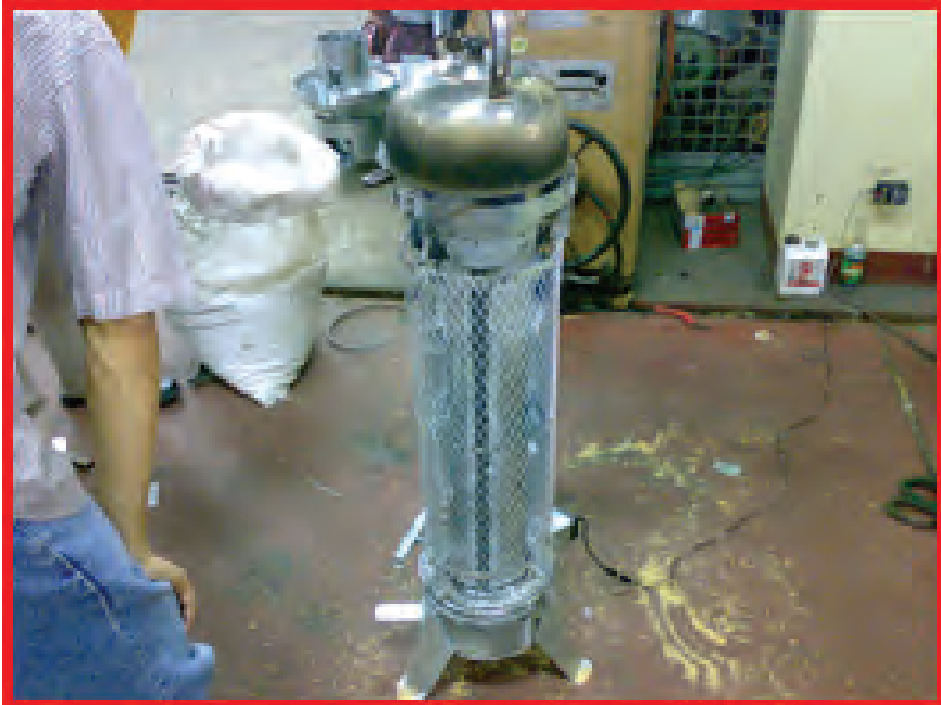
Figure 21. Batch-type rice hull gasifier stove, 14D-60 model.
