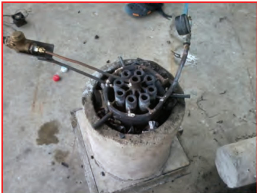
Figure 24. The instant steam generator prototype mounted on a charcoal stove.
