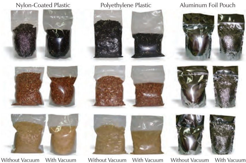
Figure 10. Ballatinao (top), Chorchoros (middle), and NSIC Rc160 in different packaging materials sealed with or without vacuum.
