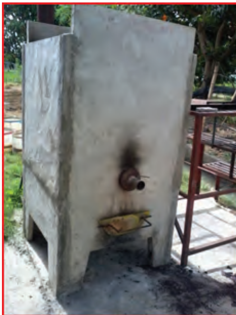
Figure 25. The continuous-type rice hull (CTRH) carbonizer made of ferrocement.
