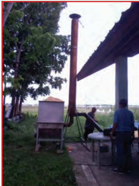
Figure 28. The carbonizer equipped with (heat recovery component) HRC during testing.
