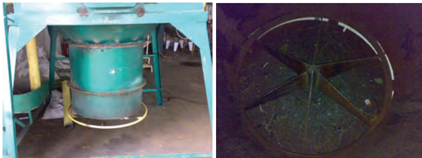
Figure 19. The 6-bladed paddle as ash discharging device.
