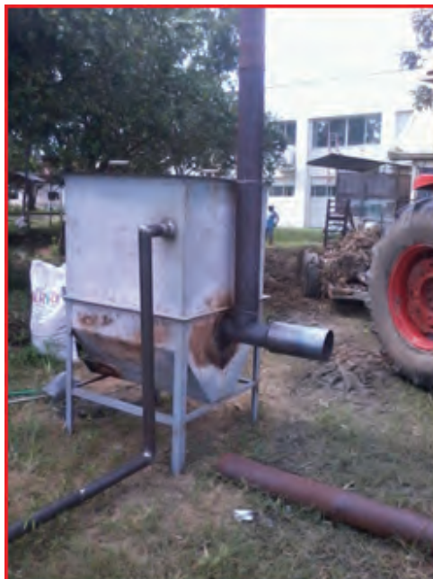
Figure 29. The continuous-type rice hull (CTRH) carbonizer equipped with line for supplying supplemental air.
