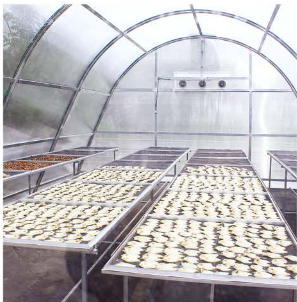
Parabola Dome Solar Dryer, an innovation from Thailand
