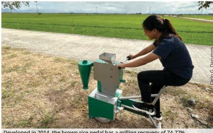
Developed in 2014, the brown rice pedal has a milling recovery of 74-77% and capacity of 1-2kg/h depending on pedaling speed.
