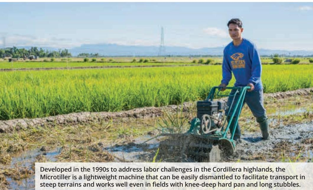
Developed in the 1990s to address labor challenges in the Cordillera highlands, the Microtiller is a lightweight machine that can be easily dismantled to facilitate transport in steep terrains and works well even in fields with knee-deep hard pan and long stubbles.
