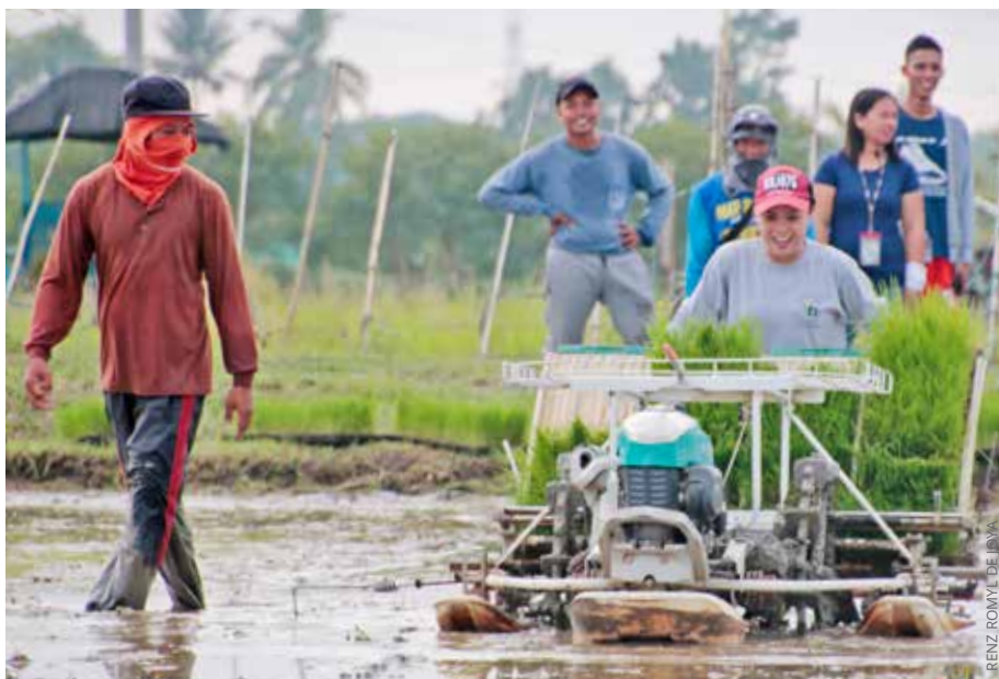
A trainee operates the mechanical transplanter during a field exercise. According to PhilRice engineer Arnold Juliano, the machine can help lessen transplanting shock in young rice seedlings, promote early seedling vigor, uniform crop stand, and enough density of seedlings per square meter.
