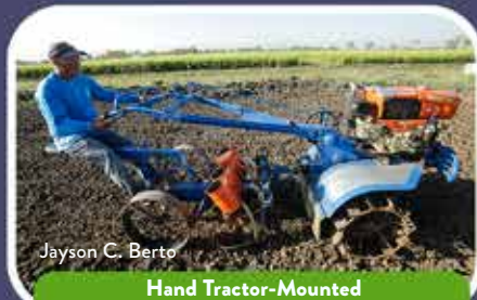
Hand Tractor-Mounted Multi-Purpose Seeder
