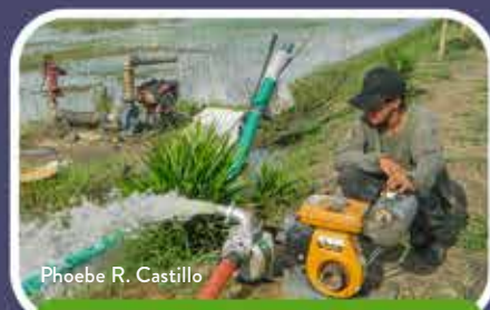
Hydrous Bioethanol Fuel-Feeding Device
