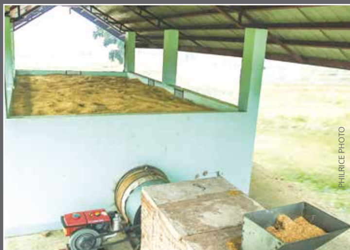
Rice hull-fuelled flat bed dryer
